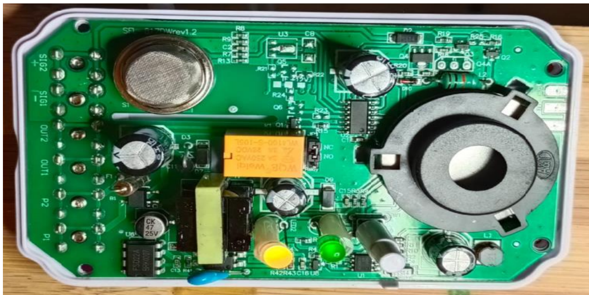
Fig. 3: The internal components assembly inside the LPG detector
