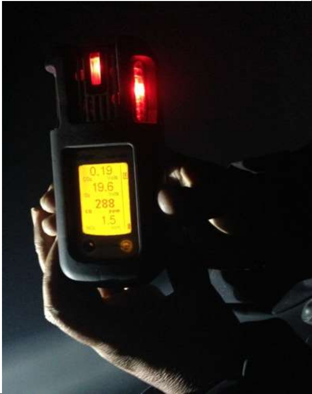
A dragger X-am 5600 gas detection meter
