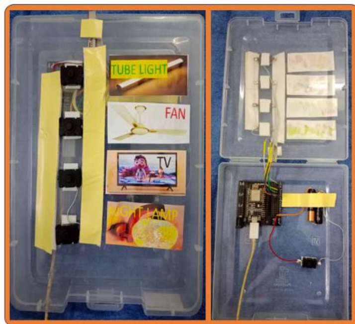
Fig. 2: Switch Board Side of the project [ Source: Author's]
