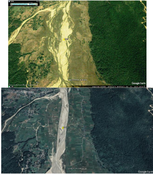
Fig. 6: River Encroachment before (2013) and after (2022) Channelization
